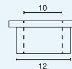
12mm hole can be reduced to 8mm or 10mm
