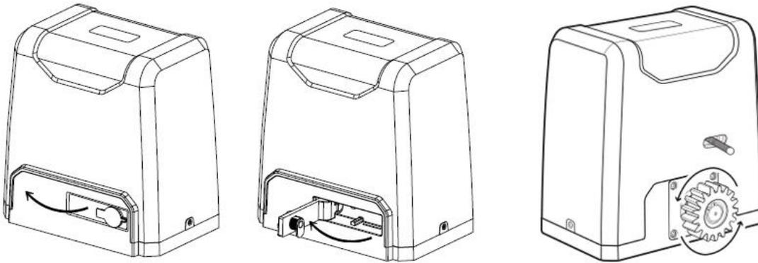
To put the gate motor into manual mode, insert the key and open the manual release bar as shown.
