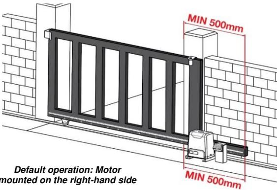
Default operation: Motor mounted on the right-hand side
