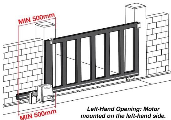
Left-Hand Opening: Motor mounted on the left-hand side.
